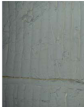
Figure 2 – Emisshield® coated Z-Blok® after 3 months in service.
